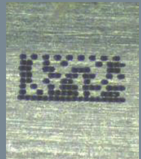
Bar codes allow full traceability for Luxeon power LEDs.
